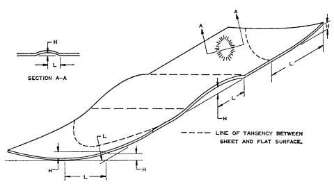
H = maximum distance between flat surface and lower surface of sheet. L = minimum distance between highest point on sheet and point of contact with flat surface. Flatness, percent = (H/L) × 100
